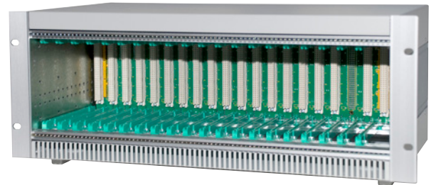
Customised 3U/4U, 19" rack-mounting Eurotec caseframe with integrated VME backplane & guides - railway application.
